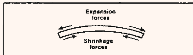
Fig. 6 Forces which cause down warp.
